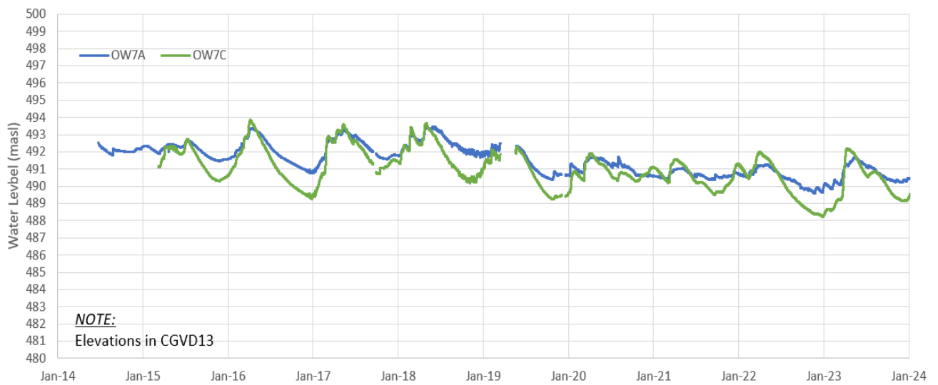
Figure B.8: Hydrograph of water levels at Well Nest OW7, in masl.
